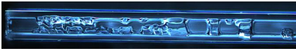
Figure 9: Side view of the hydrophilic capillary after drying of a Calcium sulfate solution plus citric acid.
