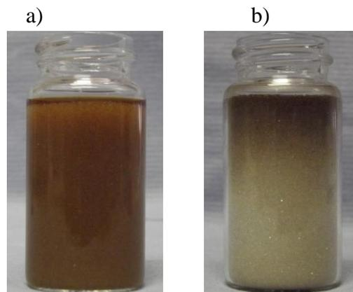
FIG. 1. (Color online) Porous medium made of  $257 (+/- 9) \mu\text{m}$  sodiocalcic glass beads packing (from *CVP Abrasif & Broyage*, cleaned with NaOH and deionized water, volume fraction: 60.3%) homogeneously filled with a coffee suspension (3.5% weight in water) before (a, beads, water, coffee) and after (b, beads, coffee) drying under natural room convection and ambient temperature.
